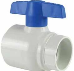
A high quality, economical quarter-turn shutoff valve designed for irrigation, pool and spa, and general purpose applications. IPS sizes 1/2" - 2" available in PVC White, PVC Gray or CPVC with socket or threaded end connectors. Sizes 3" - 4" available in PVC White with socket or threaded end connectors. 6" size available in PVC White with socket end connectors and highefficiency lever style handle for easier operation.
